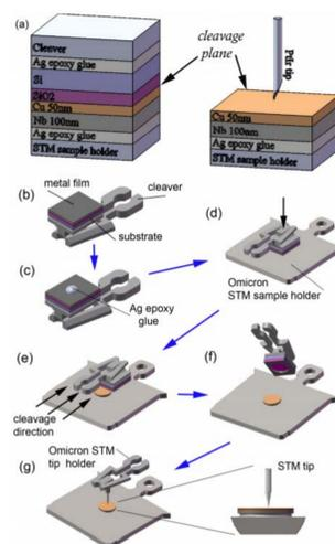
(a) - a schematic representation of the sample before and after cleaving and STM tip orientation; (b-g) - schematic cleaving process
