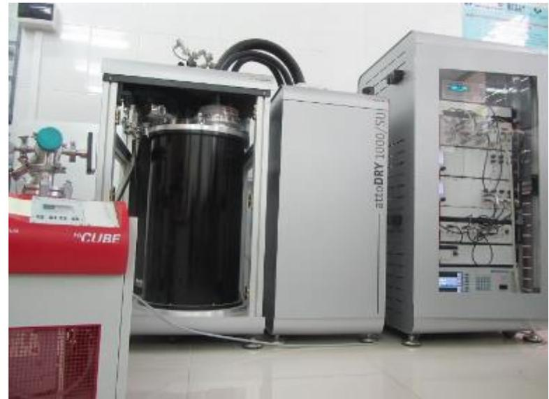
**Cryogenic system AFM/MFM AttoDRY1000**
